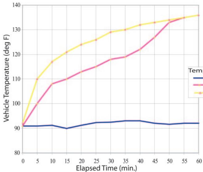
Fig 4. Interior vehicle temperature over time: closed versus cracked windows.
